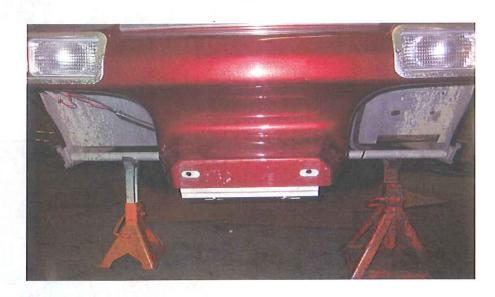
Step 2: Place Upper tower/Shock Mount plate on top of frame rails, over existing holes.
