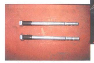
Step 5: Place two 3/8 x 4 1/4" bolts through the carrier, place two spacers over bolts. Next push bolts through the tower plate on top of frame rails and place 3/8 Nylock on end.
