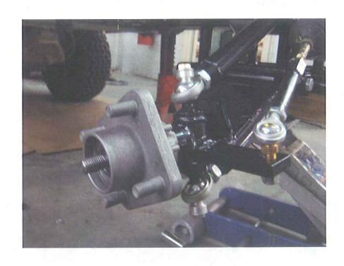
Step 9: Place new steering shaft on the end of existing steering column. Next attach opposite end to steering rack on the carrier. Tighten both bolts.
