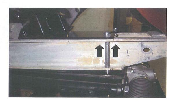
Step 7: Insert tie rods into corresponding spindle arm and place 7/16" nylock on bottom side. Repeat this step for both sides.
