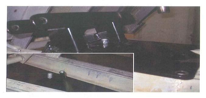
Step 6: Line up front carrier bolts (Step 4) with existing frame rail and tower plate holes. (Tape not shown in picture.) Place 3/8 Nylock on end and tighten all four nuts tower plate.
