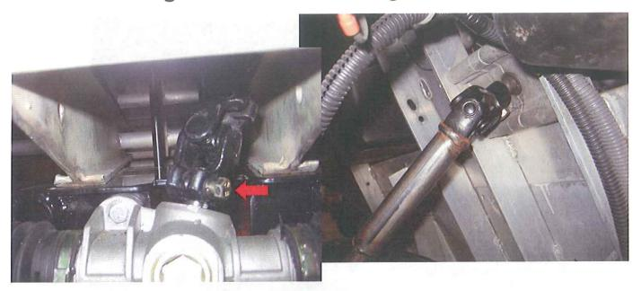
Step 10: Attach new shocks starting with lower arm on the carrier, make sure to use spacers indicated with red arrows.
