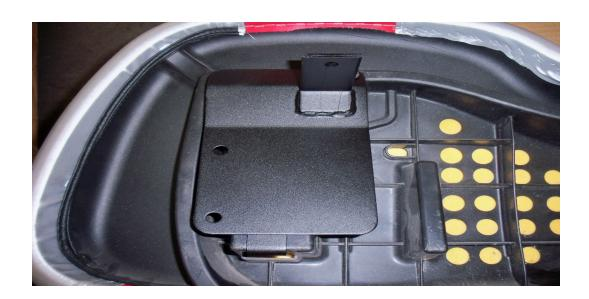
Step 8: Install front seat back brackets to seat back cushion with original bolts (Fig. 8)
