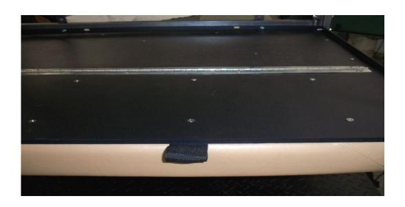
Step 11: Install rear seat back to brackets with 1/4" X 1" bolts & washers. Install seat back to seat frame with 1/4" X 1 3/4" bolts, washers, & nyloc nuts (Fig 11)
