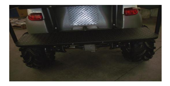
Step 6: Install step plate with 5/16" X 2" & 5/16" X 2 1/2" bolts, washers & nuts (Fig.6)
