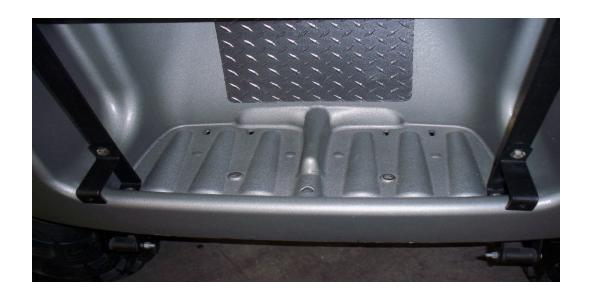
Step 2: Install seat frame braces in bag well with 5/16" X 1 1/2" bolts, washers & nuts. Install step plate brackets to frame brackets with 5/16" x 1" bolts, washers & nuts (Fig.2)
