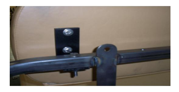
Step 10: Install front seat back brackets with 1/4" X 1" bolts & washers to seat back cushion. Install cushion to seat frame with 1/4" X 1 3/4" bolts, washers & nyloc nuts (Fig10)
