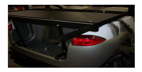
Step 3: Install seat frame with 5/16" X 1" bolts, washers & nuts (Fig. 3)
