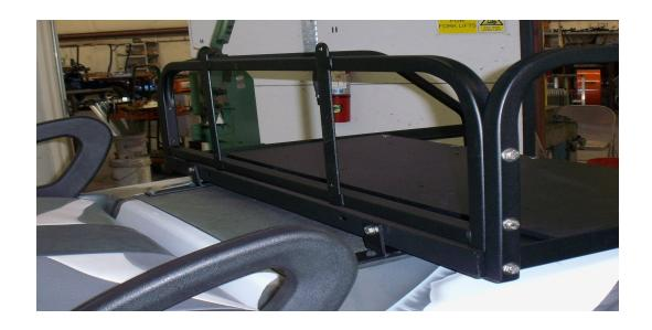
Step 5: Install seat back frame with 5/16" X 2 1/2" bolts, washers, & nuts (Fig. 5)
