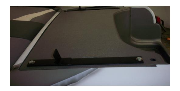
Step 1: Install seat frame brackets to cart deck with 8 MM X 25 MM bolts & washers (Fig.1)
