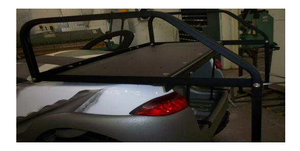
Step 4: Install side rails with 5/16" X 1 1/2" bolts, washers & nuts (Fig.4) Note: Rear bolts use acorn nuts
