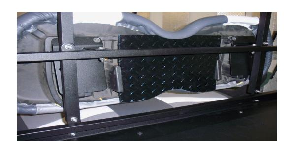
Step 9: Install seat back cushions with 1/4" X 1 3/4" bolts, washers & nuts (Fig.9)
